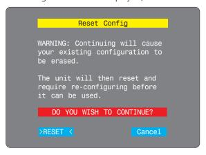
4 The CPU IP will reset and then display the first of the four <u>initial</u> <u>configuration screens</u>.
